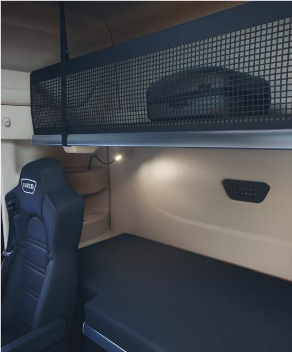
Choose from the Smart or Comfort upper bunk, which can be used as a luggage compartment or a passenger bed.
